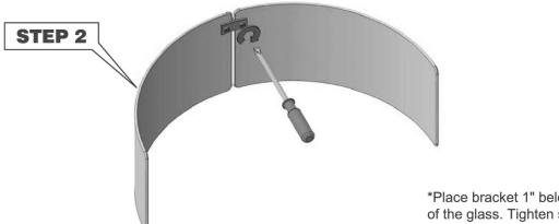
\*Place bracket 1" below the top edge of the glass. Tighten set-screws until snug. DO NOT over tighten as glass may break.
