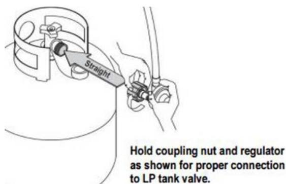
When connecting the regulator to the tank valve, make sure the coupling nut does not cross-thread on the tank valve. Cross-threading the regulator nut to the tank valve may cause a leak.
